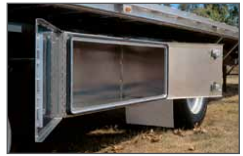
The Aero ® double door design, features no center post for ease of loading and unloading, with dual T-handle keyed locks.
