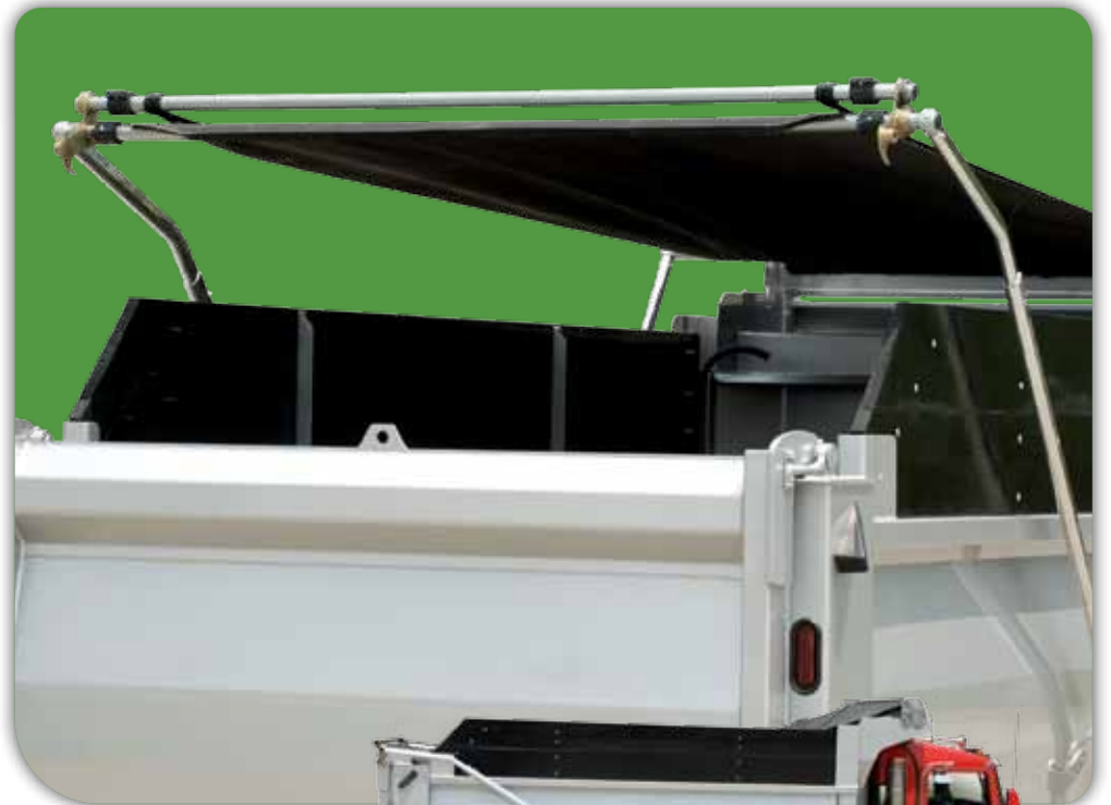
The Claw tarp hold down automatically latches & unlatches
