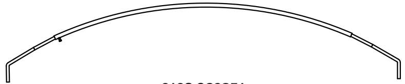
0108-960251 Adjustable Bow Assembly Steel 12"-16" Rise and 93"-103" Center To Center
