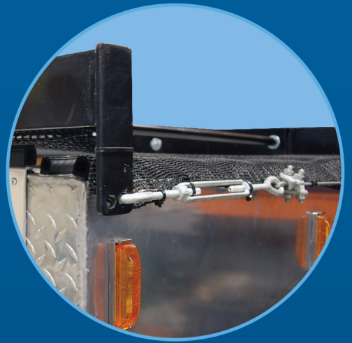
OPPOSITE SIDE hinged cable guides bring tarp over top rail
