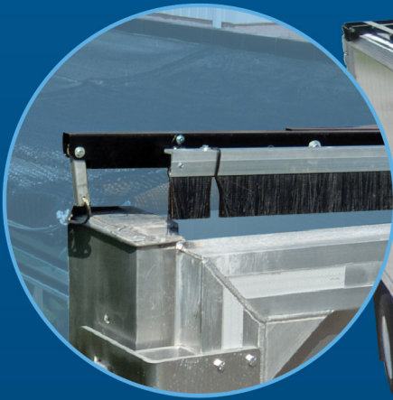
REAR adjustable brush against tailgate
